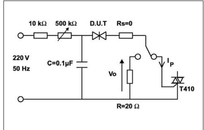
Diagram 2. Test circuit
